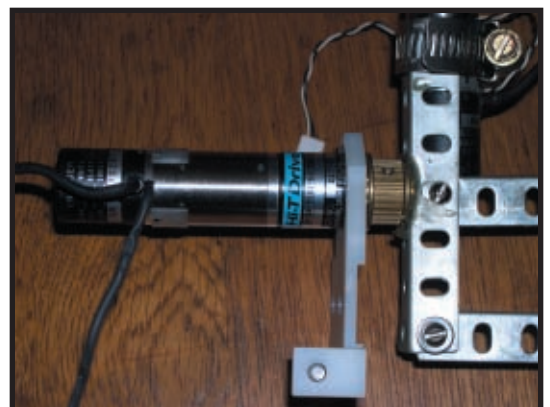
Photo 3 —The RH-5A-5502 geared DC motor is a very powerful low-voltage (5 V) geared motor that also has a 100-CPR optical encoder attached to the motor's shaft.
