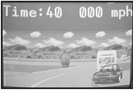
Photo 4 —Keep your eyes on the road and your hands upon the wheel. “X-Racer” (by Hydra Demo Coders Team members Jay T. Cook and Remi Veilleux) spins up the Propeller with fancy 3-D graphics techniques, such as ray casting and sprite scaling. Not bad for a chip that does everything (graphics, video, audio, gamepad, and the game itself) with just 64 KB of memory.
